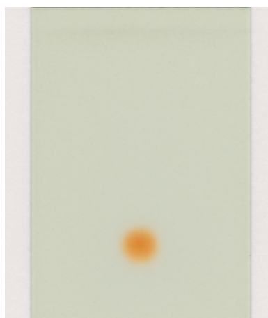
Fig. 1. Citral. The mobile phase consisted of hexane-ethyl acetate (8:2, v/v)
